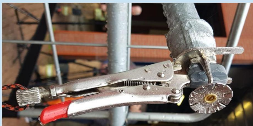
Figure 4.5 Sprinkler clamp on sprinkler head (Source TBO VRR/VRZH)
